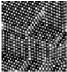
Atoms of silicon spacing ~tenths of nm
